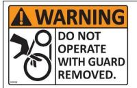
ENSURE SAFETY GUARDS ARE IN PLACE. MACHINE MUST NOT BE OPERATED WITHOUT GUARDS.
