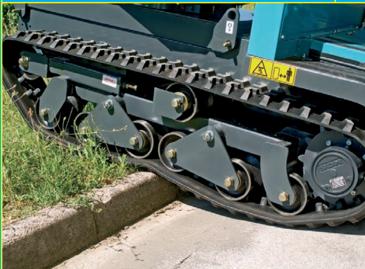
Details of the track swing / Detail Raupenschwungung /
